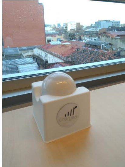
Figure 15: Photo of ChArGED 4-in-1 sensor deployed in ICAEN office floor plan
