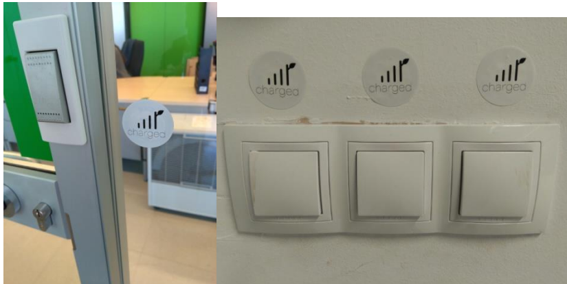
Figure 16: Photos of NFC stickers deployed at ICAEN office floor plan near lighting control switches
