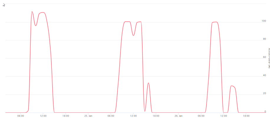
Figure 44: A/C electricity consumption measurements
