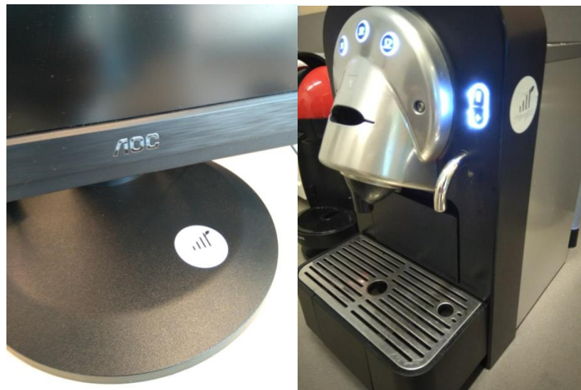
Figure 17: Photos of NFC stickers installed near computing and kitchen equipment at ICAEN office to allow users to inform the system when equipment is switch off for energy saving purposes
